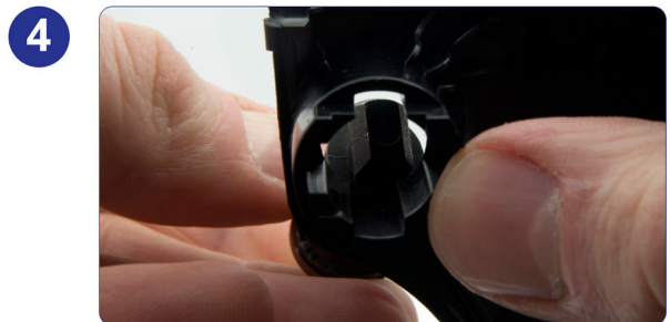
4 You need to push the lock barrel as far as you can with your thumb.
