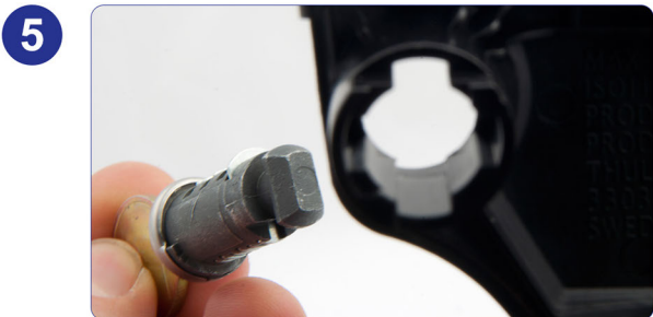
5 Using your other hand take hold of the key and remove the lock.
