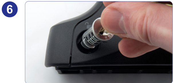
6 Place the lock barrel at a 45 degree angle into the housing.
