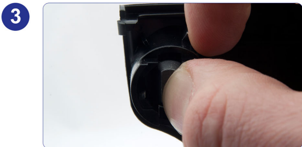
3 Keeping your finger on the lock tooth, use your thumb to push the lock barrel.
