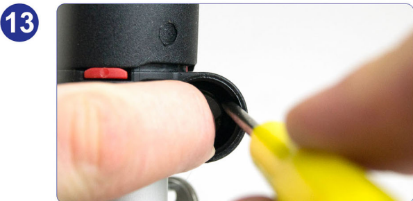
Keeping the tooth pushed in, use a finger or thumb on the other hand to push the lock barrel half way out of the housing (until the retaining tooth is free).
