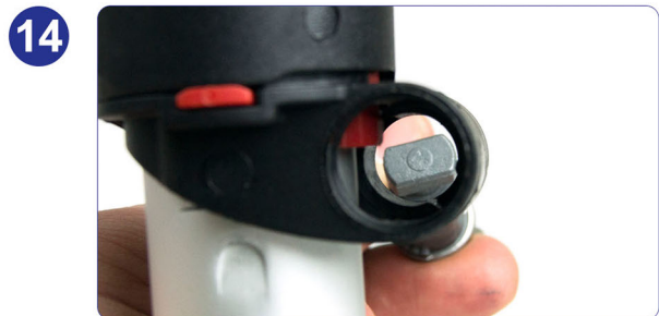
Remove the screwdriver and with the other hand remove the lock barrel (turning the barrel from left to right when removing will help).
