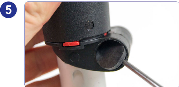
5 Once inserted to roughly 5mm, push against the lock housing in order to lever the rubber stopper out.
