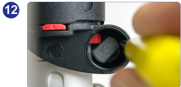
Insert a very thin flat head screwdriver into the lock housing and push the retaining tooth into the lock barrel.
