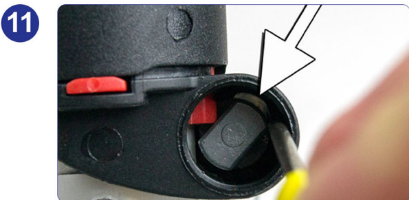
Now identify the retaining lock barrel tooth.
