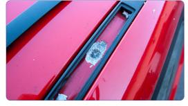
Once the covering layer of putty is removed, you will see the plastic fix point retaining screw.
