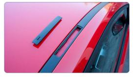
Each of the four channels are filled with a form of 'putty', the fix point is located in the centre of the channel.
