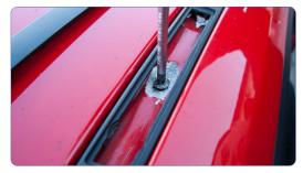
This will only unscrew to a point. Using your fingers, remove the screw.
