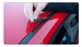
This will release the cover, lift fourty five degrees up and slide out of the housing.
