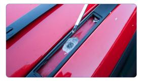
Using your philips head screw driver, remove the plastic retaining screw.
