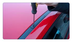
Use the flat head screw driver and turn the plastic cover screw ninety degrees.
