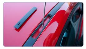
Using your flat head screw driver, begin to remove the putty from the centre of the channel.
