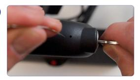
On top of the clamping handle, there is a small pre drilled hole. This accesses the lock barrel. Make sure the key is in the vertical position.
