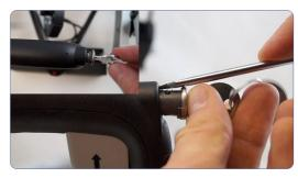
Keeping the tooth pressed down, push the lock barrel into the clamping handle just over halfway.
