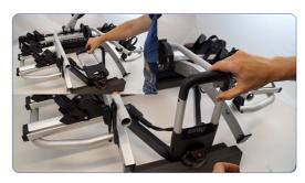
Press and hold the trigger. lift the clamping handle to the vertical position and let go of the trigger.
