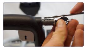
To refit the lock - you will notice one tooth on the barrel is visible. This tooth MUST be facing upwards. Have a flat head screw driver to hand.
