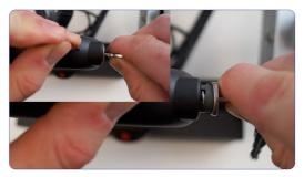
Carefully insert the straightened paper clip into the access hole and push down. Keeping the paper clip pushed down, slowly retract the lock barrel.
