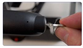
Once the lock barrel is fully inserted, the tooth will click back into place holding the lock secure.
