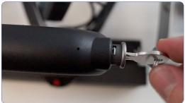
Remove the screw driver and push the lock barrel fully into the clamping handle.
