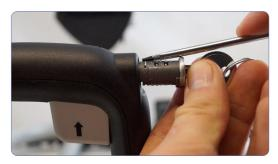
Making sure that the key is in the vertical position and the visible tooth is facing upwards, press this tooth down with the screw driver.
