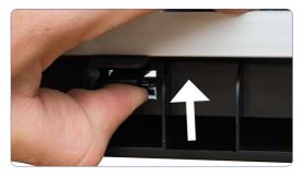
To fix the number plate into the housing you will need to pull up on each of the four retaining clips whilst pushing the number plate holder into place.
