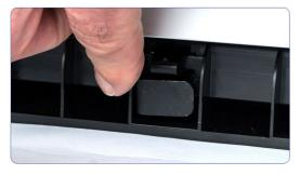
Push all four clips on the back side of the number plate down 90 degrees.
