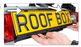
Insert both the number plate strip and number plate into the plastic housing at a 45 degree angle. Make sure both plastic catches are visible.
